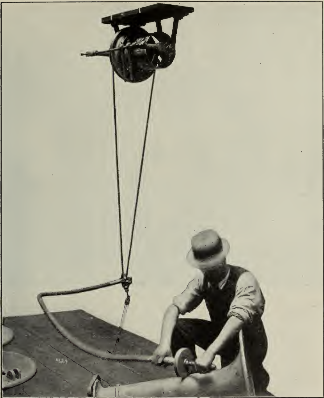
CLEANING CASTINGS WITH ABRASIVE WHEEL DRIVEN BY STOW FLEXIBLE SHAFTING.
